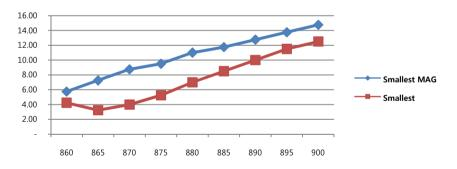
•SMALLEST MAG reads up to 1.5 meters on metal, 40% shorter than SMALLEST. Its read performance varies upon tag location, orientation, direction, RF environments, etc.
